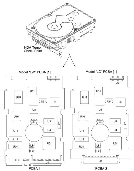
Figure 11. Locations of PCBA components listed in Table 3
