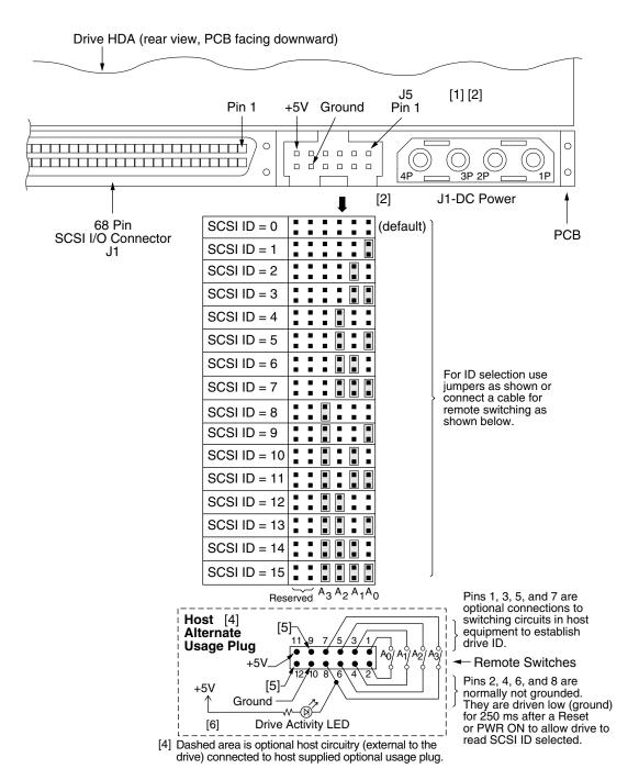
Figure 16. J5 jumper header (on LW models only)
