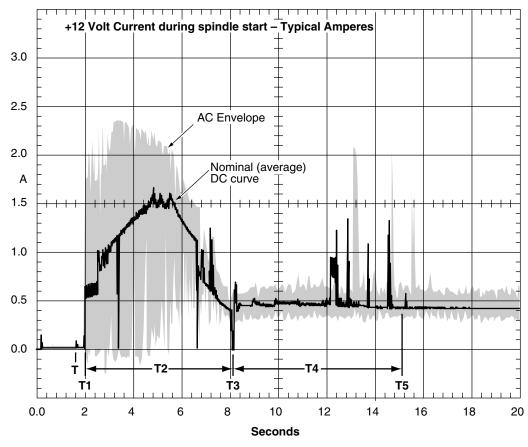
Figure 3. Typical ST318404 drive +12 V current profile
