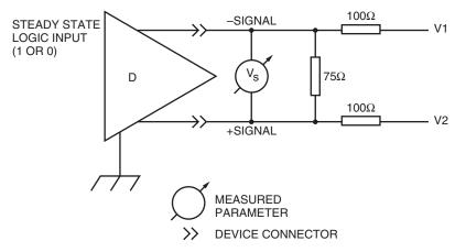
Figure 24. LVD output signals
