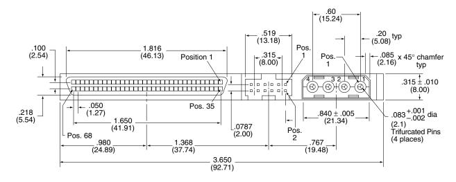
Figure 22. Nonshielded 68 pin SCSI device connector used on LW drives
