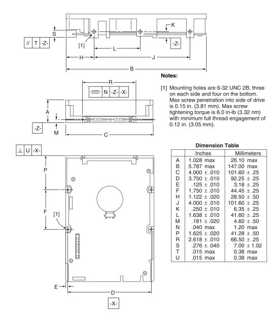
Figure 14. ST318404LC mounting configuration dimensions
