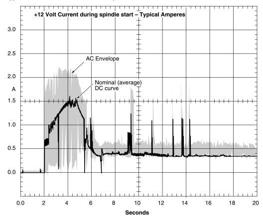
Figure 4. Typical ST39204 drive +12 V current profile
